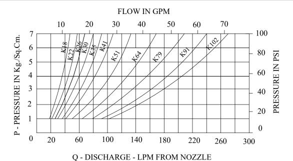
Q = K  $\sqrt{P}$  where P is supply pressure in Kg/sq.cm., K= nozzle constant (K-factor) in metric US K factor = Metric K factor MK  $\div$  14.2745
