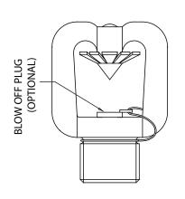
The nozzles must be hand tightened into the fitting. After hand tightening use Nozzle Wrench-NW-M for wrench tightening in to nozzle fittings. Excessive tightening torque may result into serious damage to nozzle arms and the deflector, which may affect spray pattern of the nozzle and its performance.
