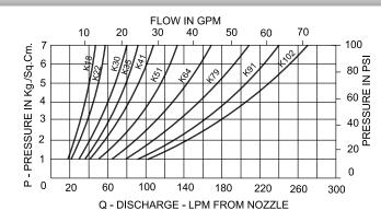
Q =K  $\sqrt{P}$  where P is supply pressure in Kg/sq.cm., K= nozzle constant (K-factor) in metric US K factor = Metric K factor MK  $\div$  14.2745
