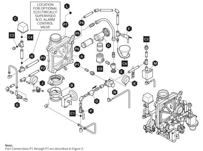
FIGURE 16 DV-5<sub>A</sub> VALVE
