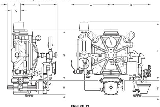
FIGURE 13 DV-5A VALVE DELUGE WET PILOT ACTUATION TRIM ASSEMBLY NOMINAL DIMENSIONS
