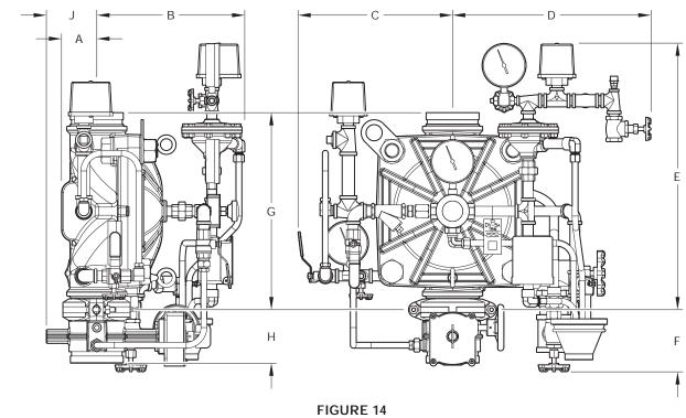
FIGURE 14 DV-5A VALVE DELUGE DRY PILOT ACTUATION TRIM ASSEMBLY NOMINAL DIMENSIONS
