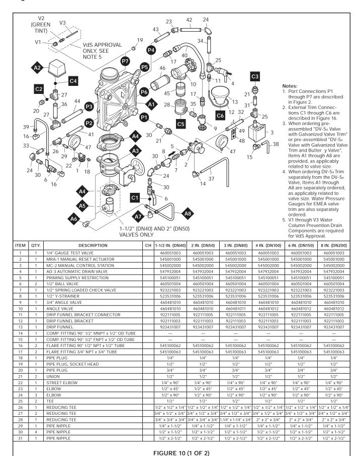
DV-5A VALVES — DELUGE WET PILOT ACTUATION TRIM — EXPLODED VIEW
