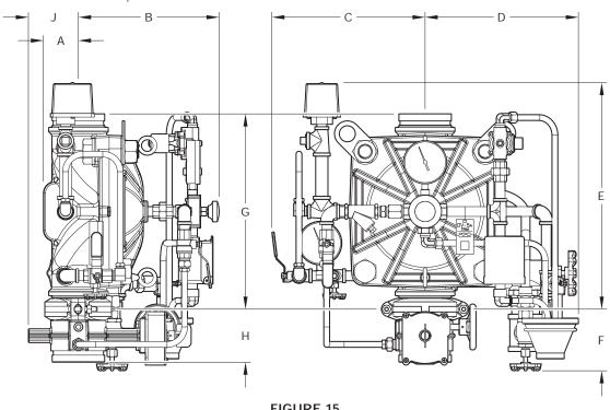
FIGURE 15 DV-5<sub>A</sub> VALVE
