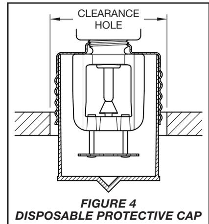
**Step 5.** Replace the Protective Cap by pushing it upwards until it bottoms out against the Support Cup. See Figure 4. The Protective Cap helps prevent damage to the Deflector and Arms during ceiling installation and/or finish. You can also use the Protective Cap to locate the center of the clearance hole by gently pushing the ceiling material up against the center point of the Protective Cap.
