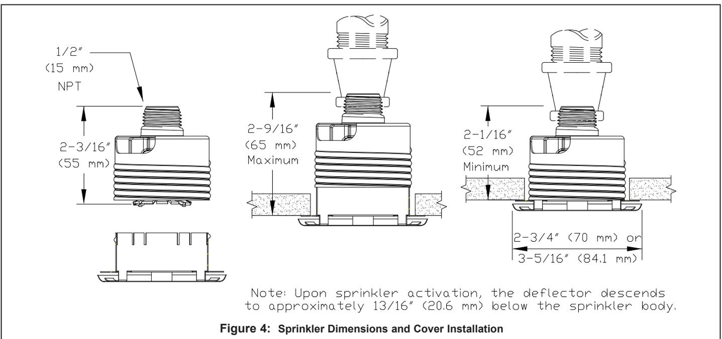
Figure 4: Sprinkler Dimensions and Cover Installation
