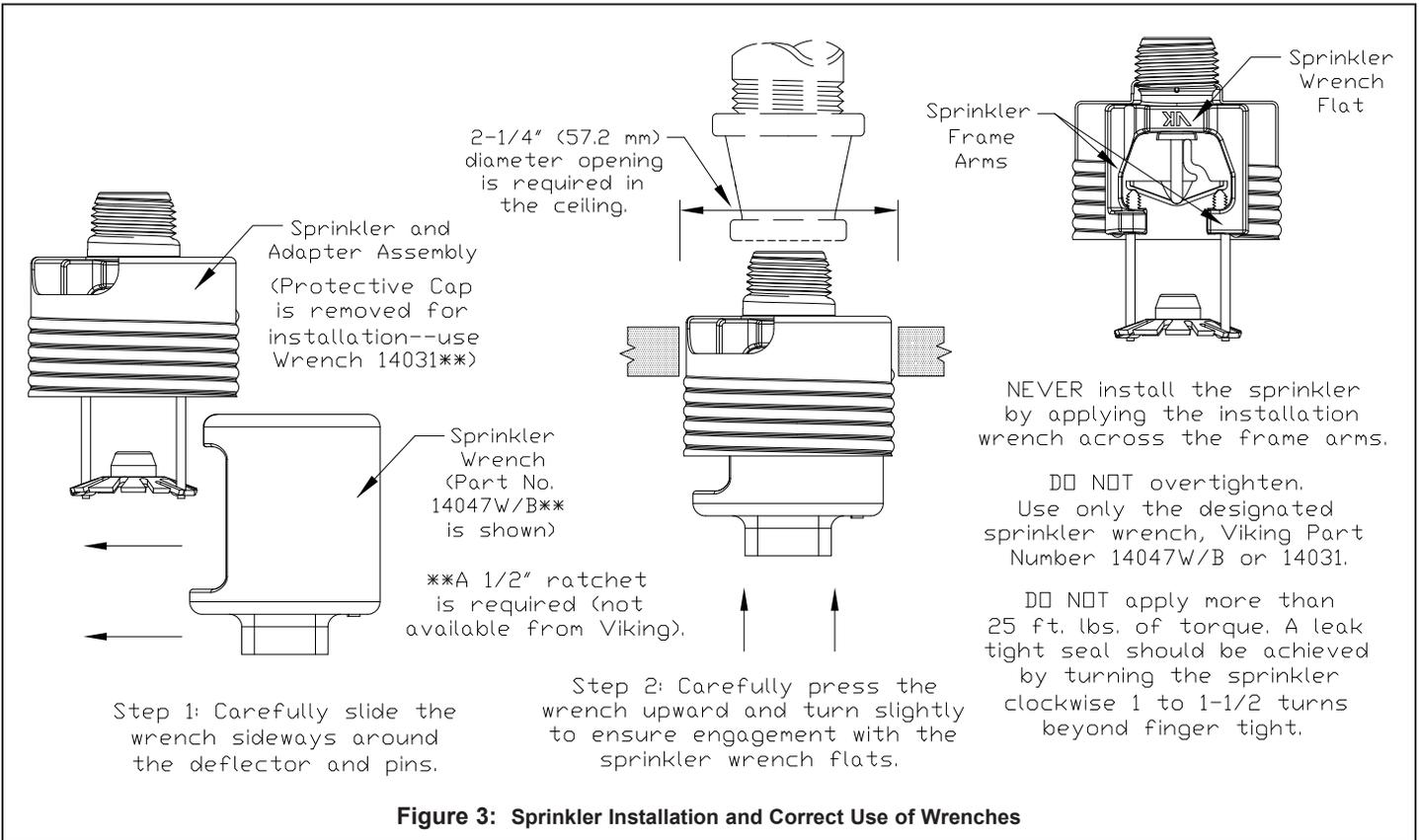
Figure 3: Sprinkler Installation and Correct Use of Wrenches
