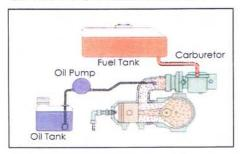
Separate Oil Filling System eliminates the need for fuel mixing.
